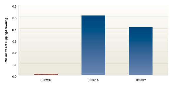
The cupping/crowning test was conducted in a temperature and humidity controlled chamber. The samples were all equalised and measured at 10% equilibrium moisture content. The chamber environment was then lifted to 16% equilibrium moisture content for a period of 10 days, producing the above results. Due to small variations in product width the test results have been standardised to a 136mm wide board. Less movement means less cupping/crowning deviation across the floor.
