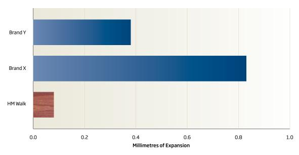
The expansion test was conducted in a temperature and humidity controlled chamber. The samples were all equalised and measured at 10% equilibrium moisture content. The chamber environment was then lifted to 16% equilibrium moisture content and the above results were recorded after 10 days. The lower the millimeters of expansion the more stable the floor. Excessive expansion leads to tenting whereby the edges of boards lift off the subfloor.
